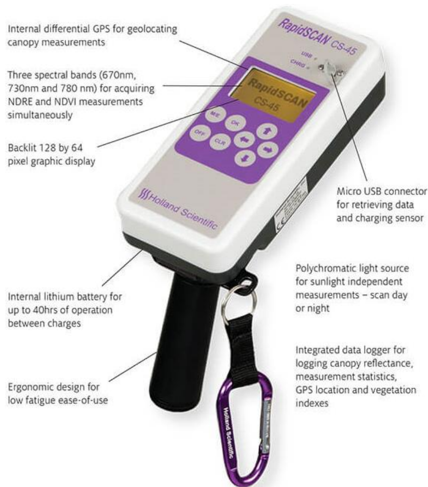
Figure 16. Equipment for measuring NDVI, the handheld RapidSCAN CS-45. Photo from Holland Scientific homepage.
