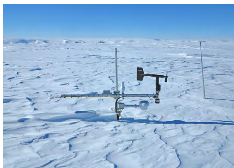
Figure 3.2 Snow cover at the summit station AWS3 had almost buried the sensors (left image) and required the boom to be raised (right image), taking advantage of the flexibility of the GEUS AWS tripod design that can accommodate an extended-length mast for sites where thick snow cover can be expected. Photos by Michele Citterio (Copyright GEUS).
