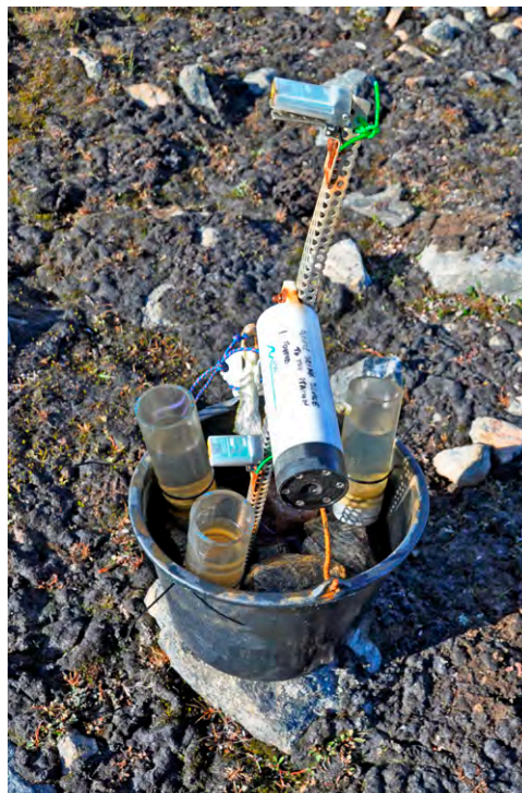
Figure 6.31 Various data loggers and other sampling devices that are placed at the lake bottom for up to 12 months. Photo: Kirsten S. Christoffersen.
