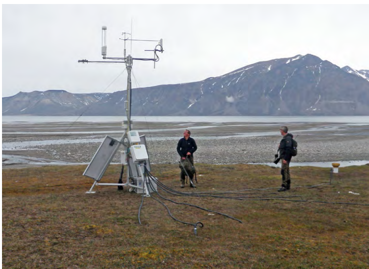
Figure 6.11. Torben R. Christensen and Marcin Jackowicz-Korczynski next to the newly installed eddy covariance system in the river Zackenberg delta, August 2014. Photo: Lau G. Petersen.
