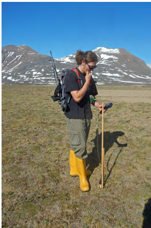
Figure 6.13 Soil moisture measurements. Photo: Alfred Wegener Institute, Germany 2014
