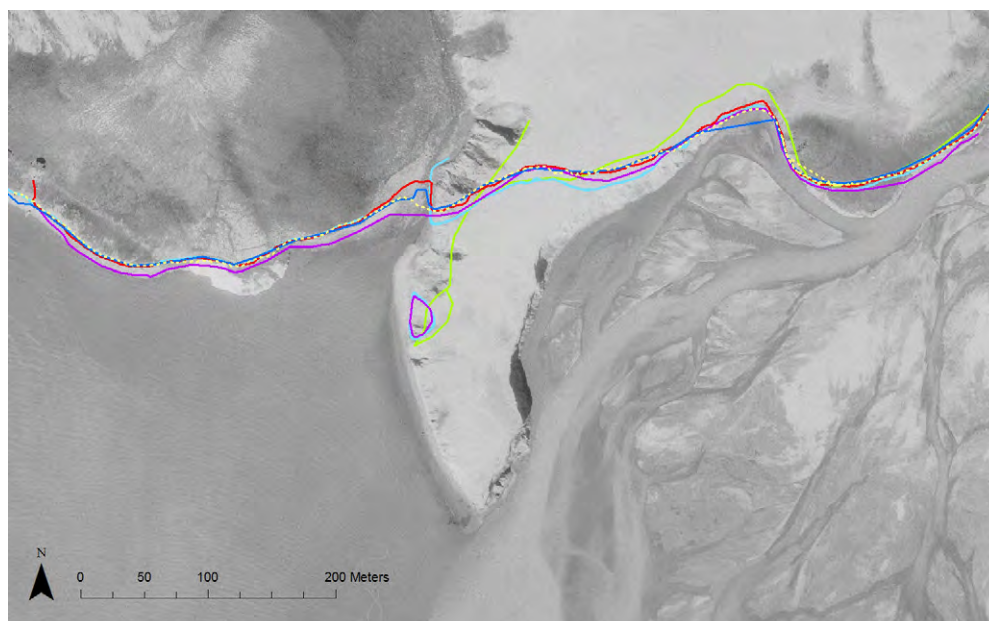
Figure 2.17 Delta- and coastal cliff line measured by DGPS in 2008 (green line), 17 October 2010 (blue line), 12 October 2011 (purple line), 28 September 2012 (red line), 10 September 2013 (dark blue line) and 8 September 2014 (dotted yellow line) on an aerial photo from 8 August 2000.
