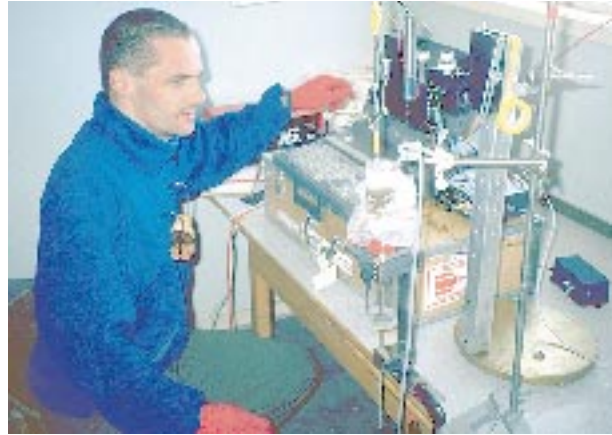
Fig. 5.2.5.1. Measurement of the oxygen concentration profile within the sediment. The measurements were performed in the laboratory of the Daneborg Weather Station.
