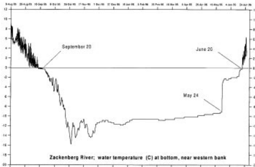
Fig. 3.2.2. Temperatures (°C) measured at the bottom of the river Zackenbergelven, 1995-1996. Autumn freeze-up and spring break-up of the river are clearly indicated.
