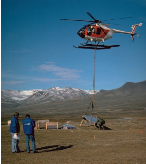
Fig. 6.2. A Hughes 500 helicopter transported 42 t of cargo from the ship to Zackenberg station in 120 sling-load flights at low level above the south part of Zackenberg-dalen.
