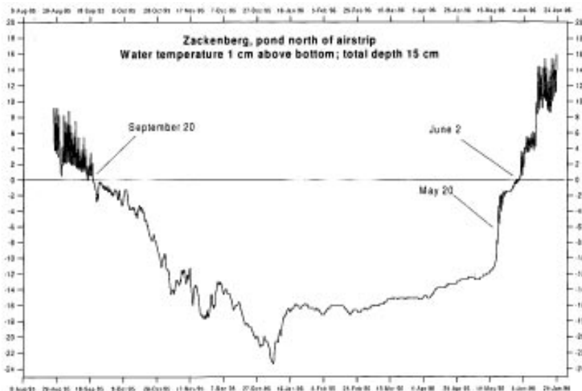
Fig. 3.2.3. Temperatures (°C) measured 1 cm above the bottom in a pond at Zackenberg, 1995-1996. Autumn freeze-up and spring thaw of the pond are clearly indicated.
