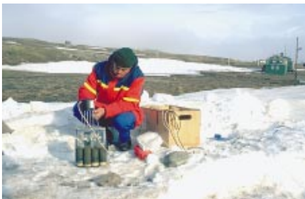
Fig. 5.2.4. Sampling from sediment cores during incubation at the end of June. In June, when ice and snow covered Young Sund, the sediment cores were submerged in bottom water from the locality and the incubator cooled with snow to maintain correct in situ temperature. Later, ice was collected from icebergs and brought to the laboratory for temperature control.
