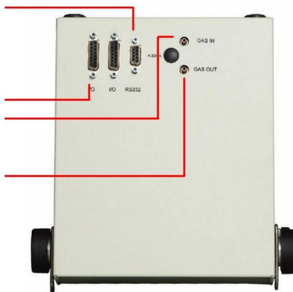
Figure 22. Upper figure shows the EGM4 which is used for measuring CO 2 concentrations. The lower figure shows the top of the instrument.
