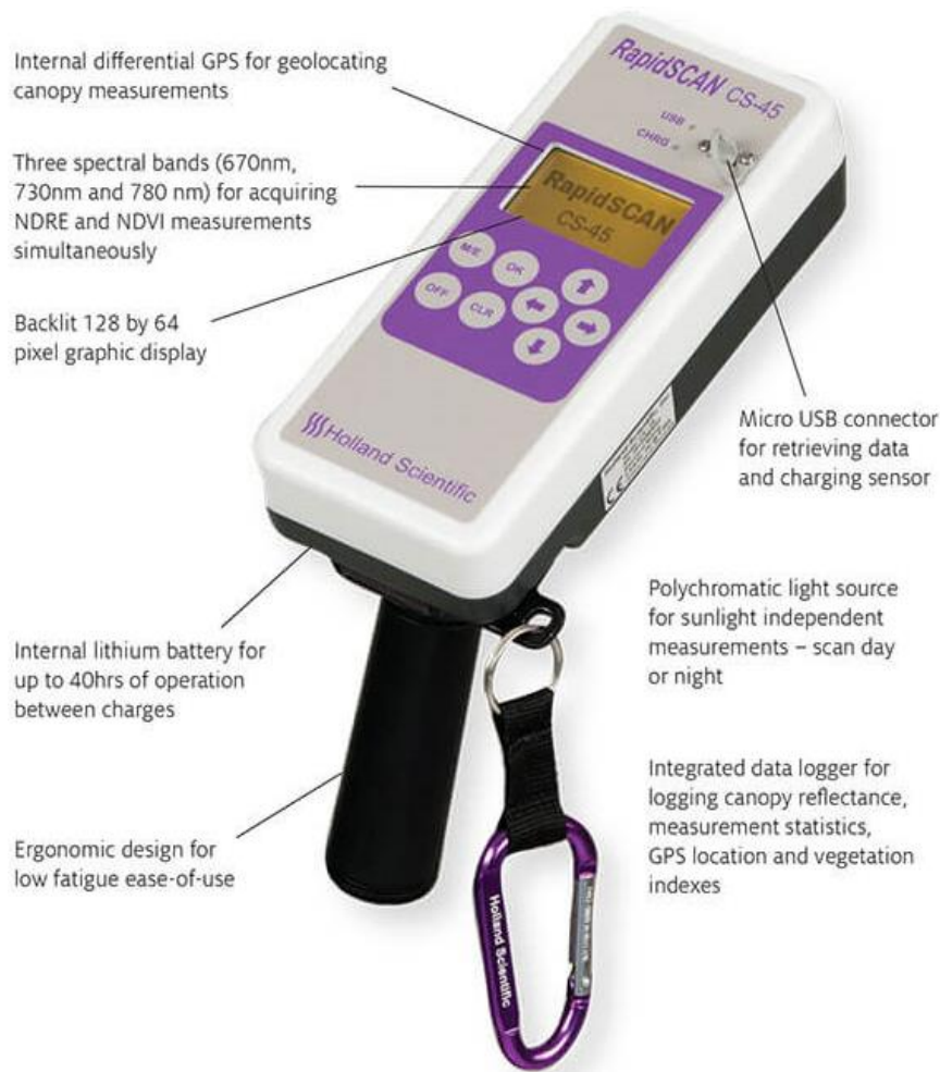
Figure 17. Equipment for measuring NDVI, the handheld RapidSCAN CS-45. Photo from Holland Scientific homepage.
