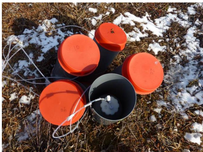
Figure 5.9 Soil water bottles hidden in grey storage tubes with red lids. Lysimeters buried in 10-50 centimeters depth.
