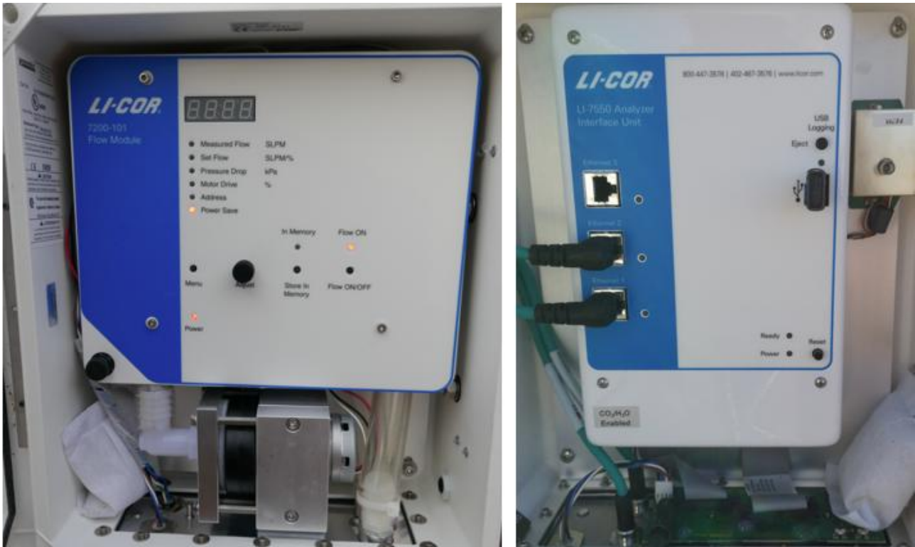
Figure 3.4 Flow module LI-7200-101 (inside Box 5 in Figure 3.2) to the left, and Licor Analyzer Interface Unit AIU LI-7550 (inside Box 6 in Figure 3.2) to the right.
