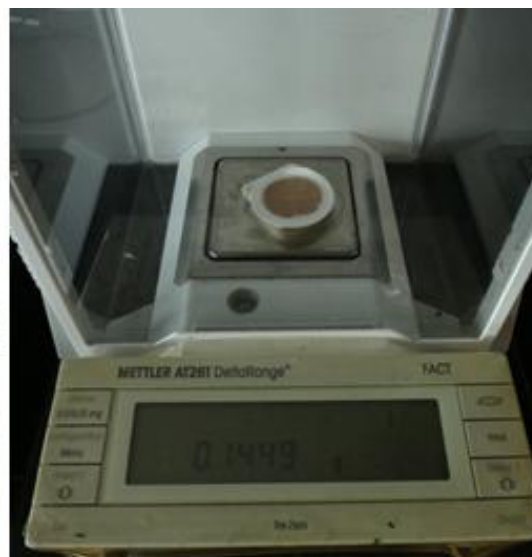
Figure 7.6 Tray of tin foil with filters -always transport them in the closed box (left). Weigh filter on a small tray on the analytical scale (right).
