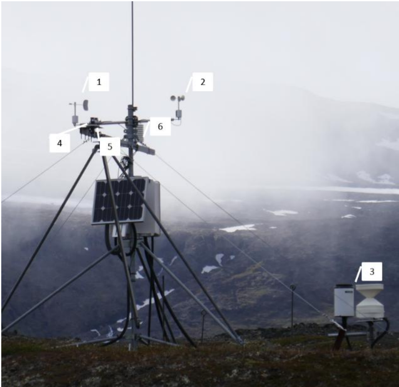
Figure 2.10 AWS3 Blæsedalen. 1) Wind direction, 2) Wind speed, 3) rain, 4) PAR, 5) NDVI, 6) Air temperature and relative humidity
