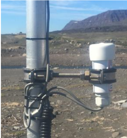
Figure 2.16. HOBOnast T4 in the delta. Looking towards west. Datalogger with protection cap that must be removed when communicating with the logger.
