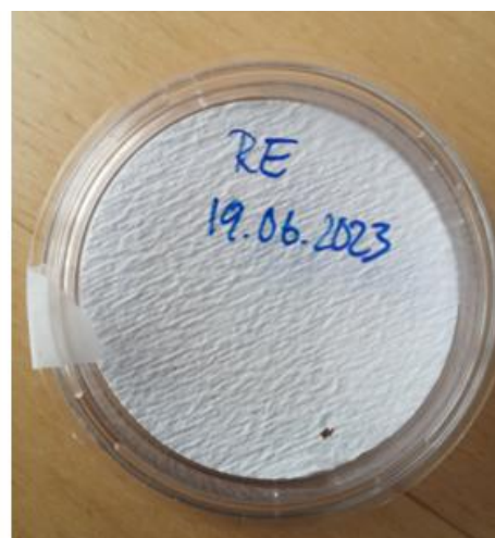
Figure 7.7 Place the dried filter in the plastic petri box. Note date and time label on the outside.
