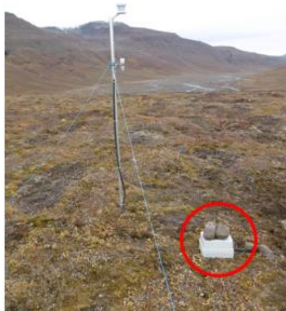
Figure 5.6.1 Tinytag dataloggers inside the grey box at T1-ground. Installation depths 30, 70, 85 cm
