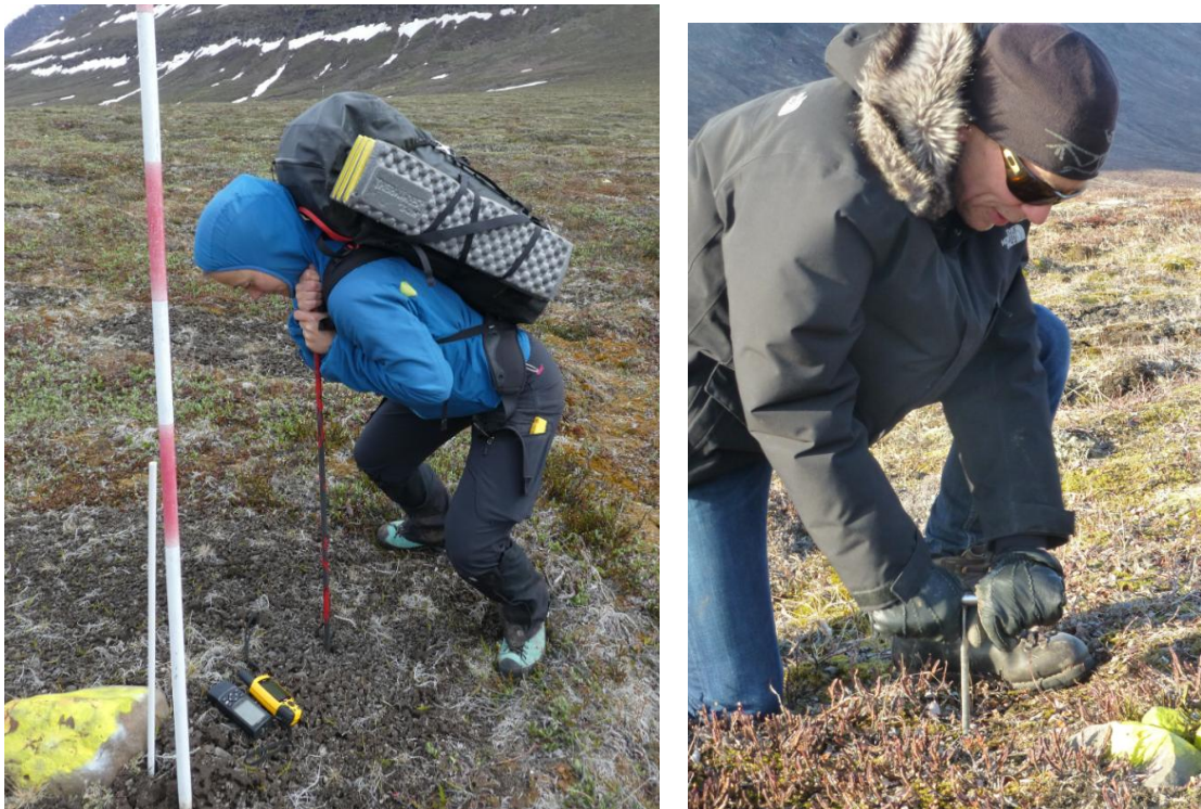
Figure 5.3. Probing the soil. A steel probe is forced vertically into the soil to reach the frozen surface.
