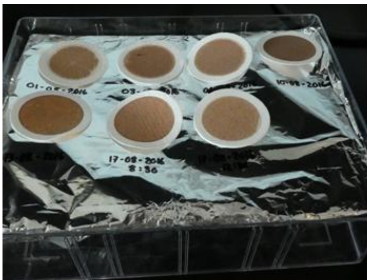
Figure 7.6 Tray of tin foil with filters -always transport them in the closed box (left). Weigh filter on a small tray on the analytical scale (right).
