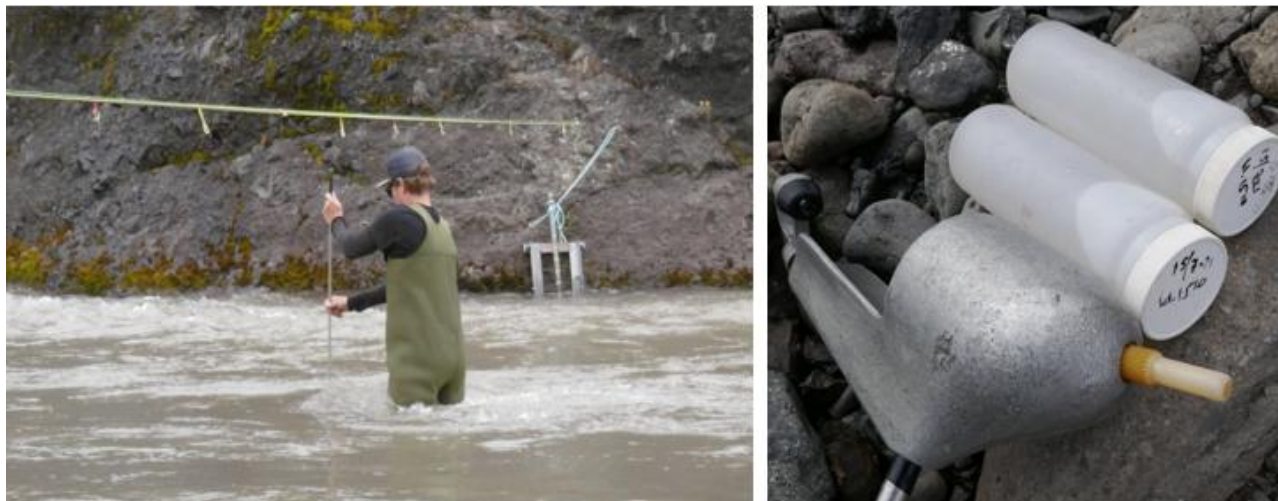
Figure 6.17. Sampling of water using depth integrating sampler USDH-48.
