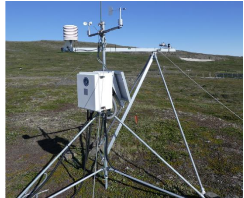
Figure 2.9 AWS3 in Blæsedalen. Looking north into Blæsedalen. The mast to the left holds the precipitation collector.
