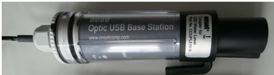
Figure 6.7 Water level sensor from HOBO Onset. The black cap is removed when communicating with the logger.
