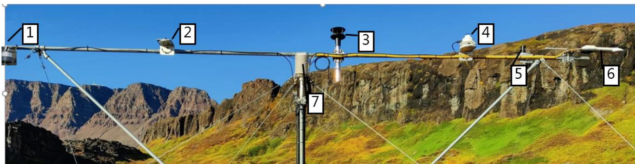
Figure 2.5 The Automatic Weather Station AWS2 in Østerlien. 1) Snow depth (SR50 Sonic sensor), 2) PAR sensor, 3) Sonic Wind direction and Wind speed, 4) UVB sensor, 5) SKYE sensor RED/NIR. 6) Net radiometer CNR4, 7) Temperature and humidity sensor.
