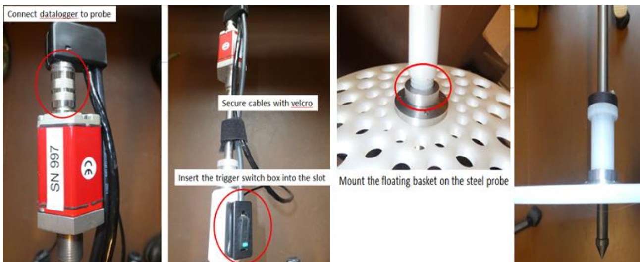
Figure 4.7 How to connect and prepare the probe.
