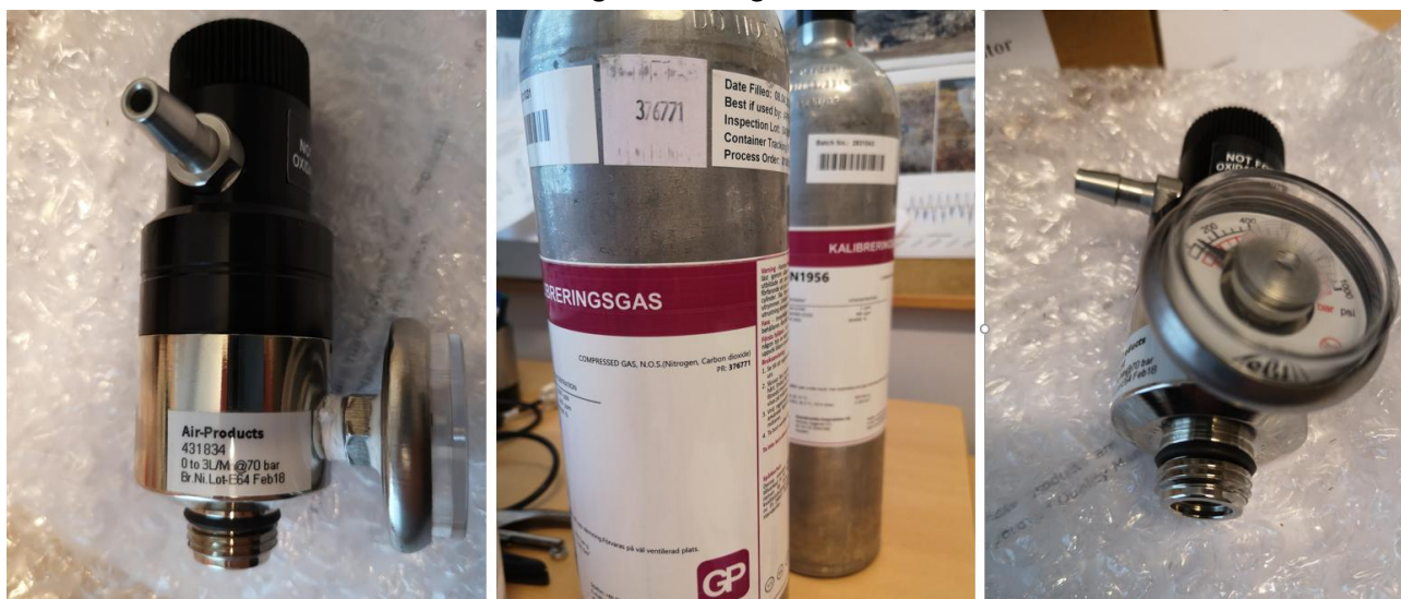
Figure 3.11. Calibration gas bottles (from 2020) and flow regulator.
