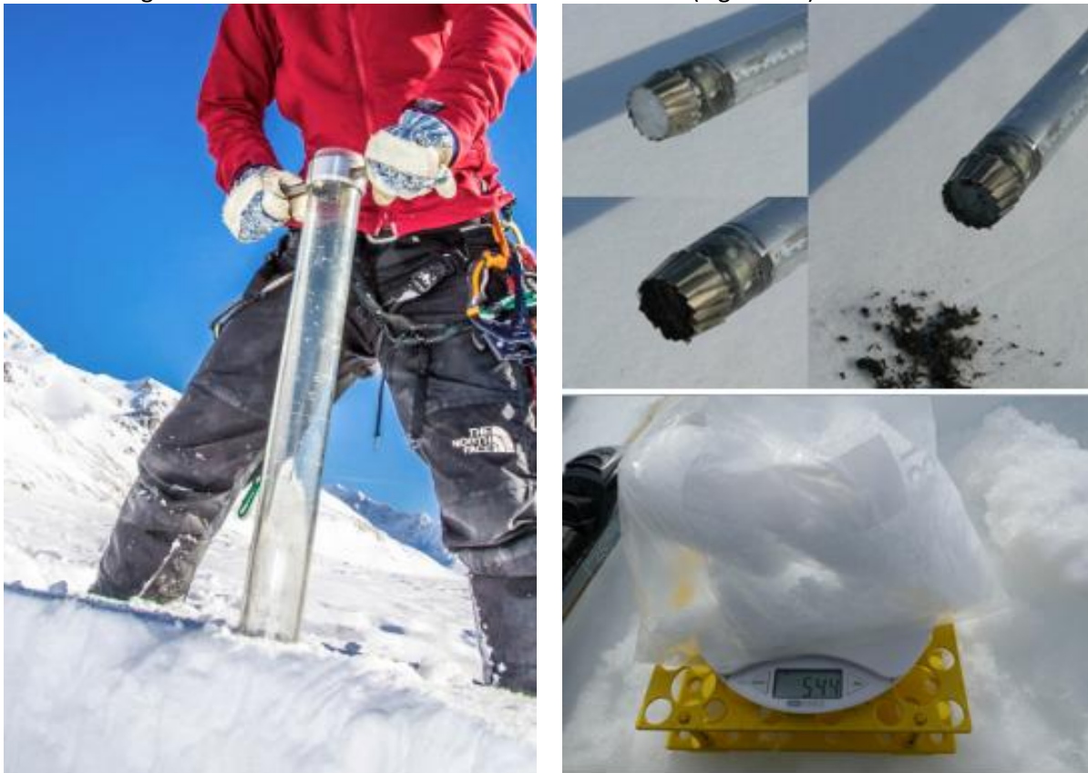
Figure 4.13 Snow sampling tube. Scale and plastic bag with snow core.
