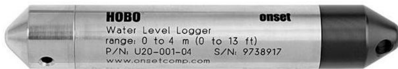
Figure 6.7 Water level sensor from HOBO Onset. The black cap is removed when communicating with the logger.
