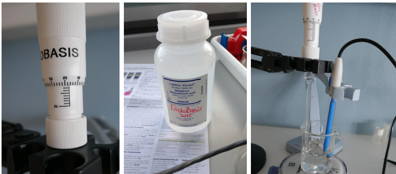
Figure 7.2 Gilmont micrometer burette –the scale can be read with 3 decimals (left). 0.01 M HCl (middle). Set-up for titration (right)
