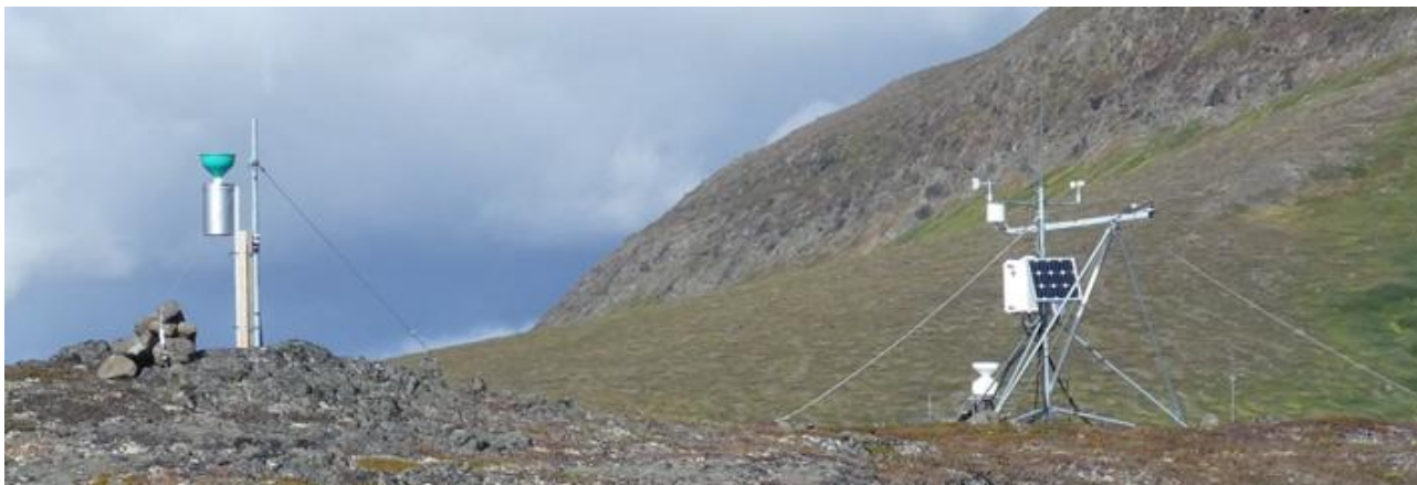
Figure 9.2 Cumulative integrated sampler (totalizer) (left) and AWS3 weather station (right).
