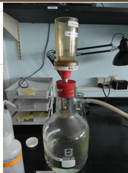
Figure 7.5 Vacuum pump. Scale to weigh the bottle when full and when empty (left). Analytical scale (middle). Set-up for filtering using the 3 L bottle (right).
