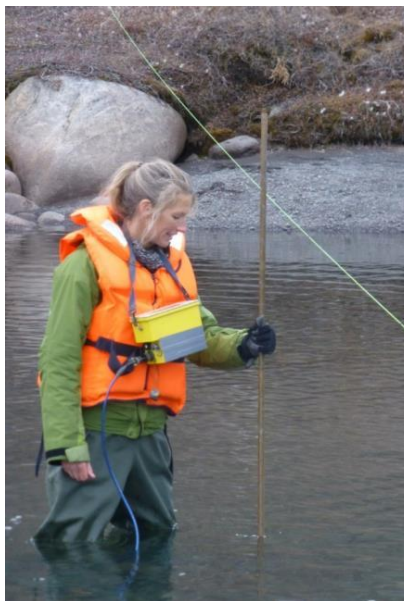
Figure 6.16 Valeport flowmeter for manual discharge measurements at shallow depth –or in smaller streams where you can easily wade across the profile.
