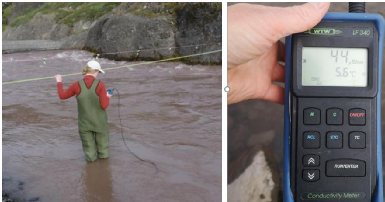
Figure 6.19. In situ measurement of conductivity and temperature in the river (left). The conductivity meter (right).
