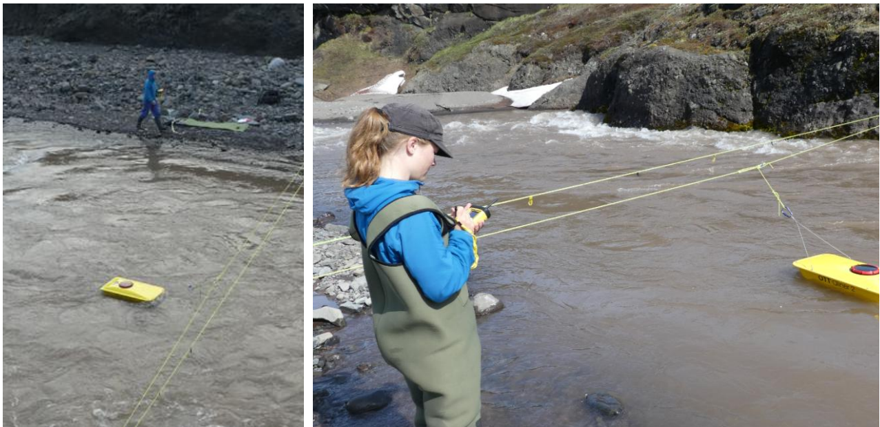
Figure 6.15. Discharge measurement carried out from the western side of the river crossing. The Q-liner boat is attached to the rope and can be pulled from one side of the river to the other. Measurements are carried out for each half meter.
