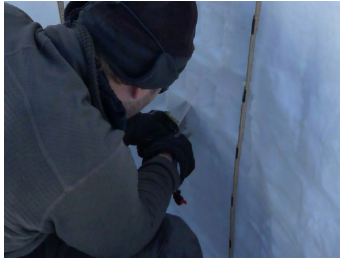
Figure 19: Demonstrated insertion of RIP cutter (vertical).
