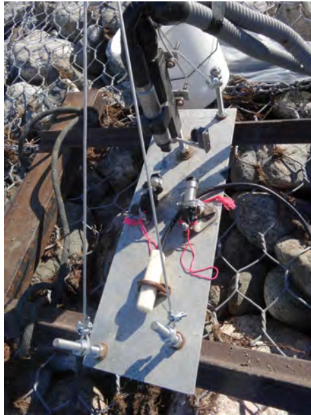
Figure 45: Metal frame for installation of OBS, diver and conductivity sensor
