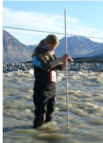
Figure 52: Standard velocity profile in the river and an example of measuring velocity at two different water depths.
