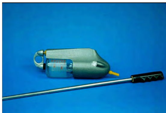
Figure 59: US DH-48 depth integrating sampler with 500 ml plastic bottles. To remove or insert the bottle; pull back and turn the handle in the back.
