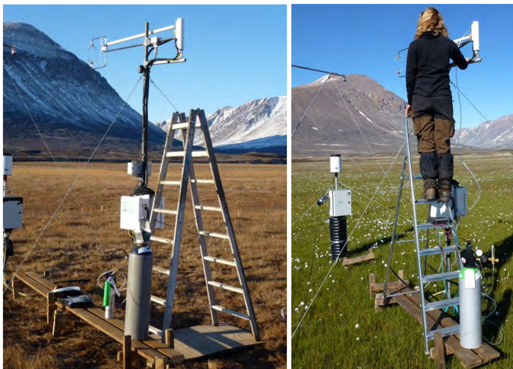
Figure 75: Setup for span testing or calibrating Licor7200. Left; the ladder is used for connecting or disconnecting the Bev-a-line tube for the air intake on the mast (where the white tube is connected to the licor house), Nitrogen and span gas, the computer is connected to the Licor7200 underneath the white enclosure using a RS232 cable. Right; calibration ‘in action’ the reference gas is connected to the licor7200 through the bev-a-line tube and in situ measurements are read from the PDA and noted in the calibration sheet.
