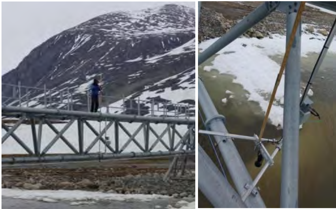
Figure 58: Lineup for levelling of the distance sensor
