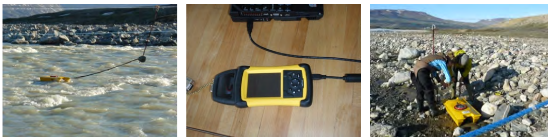
Figure 51: Q-liner boat in the river (left). PDA connected to computer (mid). Attaching the Qliner to the wire (right).
