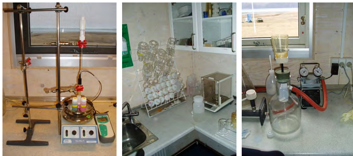
Figure 62: Laboratory in Zackenberg. pH meter next to the magnetic stirrer. The pH electrode is held by the lower clamp and the acid dispenser is held by the upper clamp (left). Analytical balance (middle). Device for filtration of water samples. Filtered water is collected directly into a clean sample bottle. Vacuum is applied by the electrical pump connected to the glass bottle (right).
