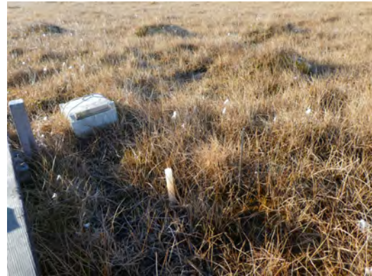
Figure 80: Looking down into the area in front of the chambers. Between the chambers there are fixed plastic probes, use the top of these to measure the active layer.
