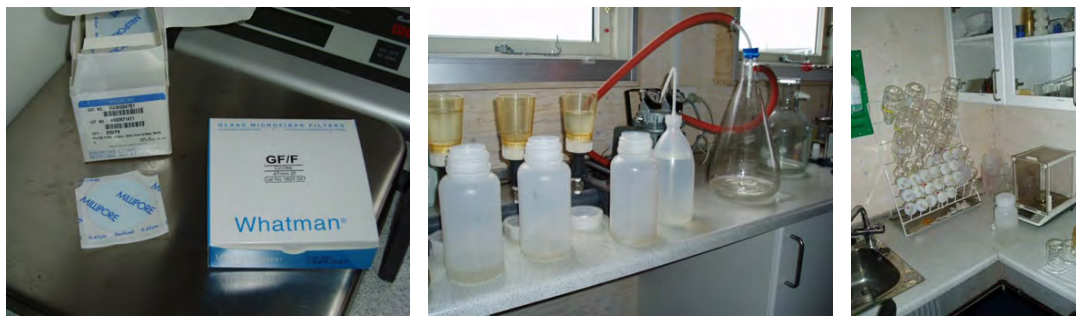
Figure 63: Whatman GF/F filters are used for filtration of suspended sediment samples (left). Milipore filter assembly connected to the vacuum pump. Three samples can be filtered at the same time (Mid). Analytical balance (right).
