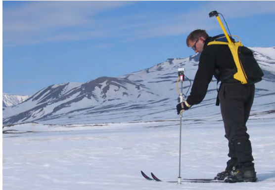
Figure 15: Magnaprobe in use. The metal probe is pushed into the snow and down to the ground surface. The floating basket moves up and down and gives the position of the snow surface. The probe is connected to a CR10x datalogger. A depth reading and a GPS position are made when you press the thumb switch on the handle.
