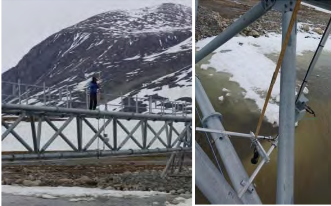
Figure 62: Lineup for levelling of the distance sensor
