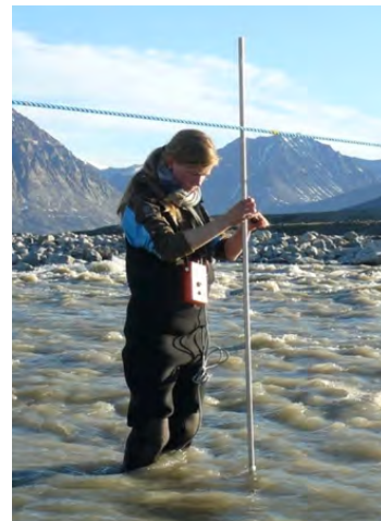
Figure 56: Standard velocity profile in the river and an example of measuring velocity at two different water depths.
