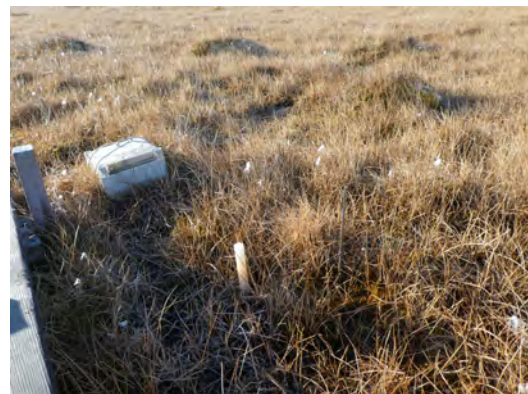
Figure 79: Looking down into the area in front of the chambers. Between the chambers there are fixed plastic probes, use the top of these to measure the active layer.
