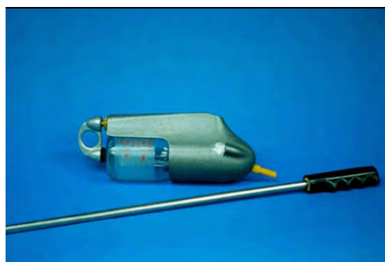
Figure 63: US DH-48 depth integrating sampler with 500 ml plastic bottles. To remove or insert the bottle; pull back and turn the handle in the back.
