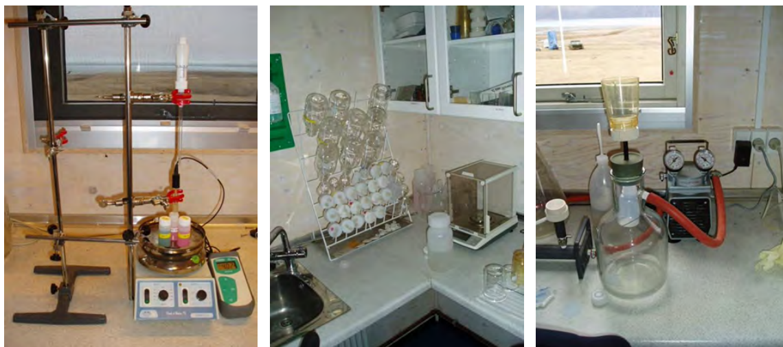
Figure 66: Laboratory in Zackenberg. pH meter next to the magnetic stirrer. The pH electrode is held by the lower clamp and the acid dispenser is held by the upper clamp (left). Analytical balance (middle). Device for filtration of water samples. Filtered water is collected directly into a clean sample bottle. Vacuum is applied by the electrical pump connected to the glass bottle (right).
