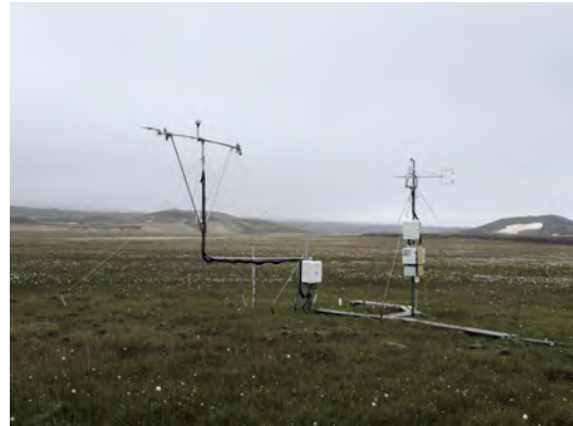
Figure 9: MM2 with energy balance mast (left) and eddy covariance tower (right).
