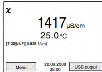
Figure 65: Display of cond3310 during measurement with nonlinear temperature compensation with a reference temperature of 25 degrees.
