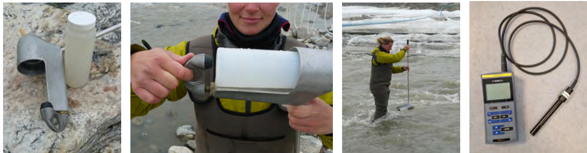
Figure 64: Depth integrating sampler and conductivity meter used during morning and evening sampling.
