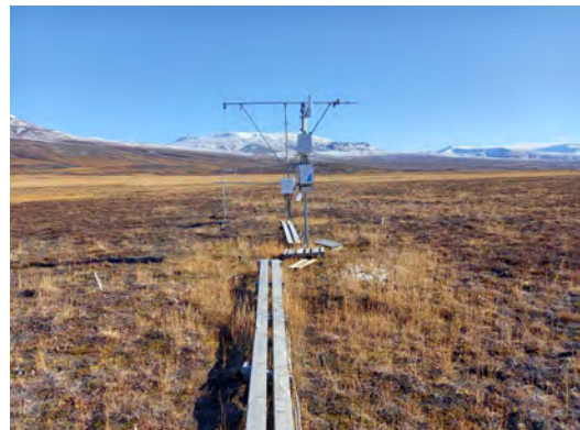
Figure 8: MM1 with energy balance mast, behind eddy covariance tower and enclosure instruments.
