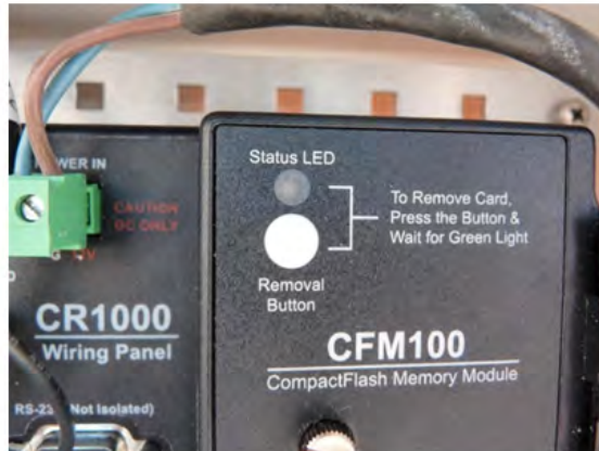
Figure 10: CFM100 Compact Flash Memory Module with diode turned off that indicates the CF card is ok (as on picture). If the Status LED is orange then the CF card is NOT working.
