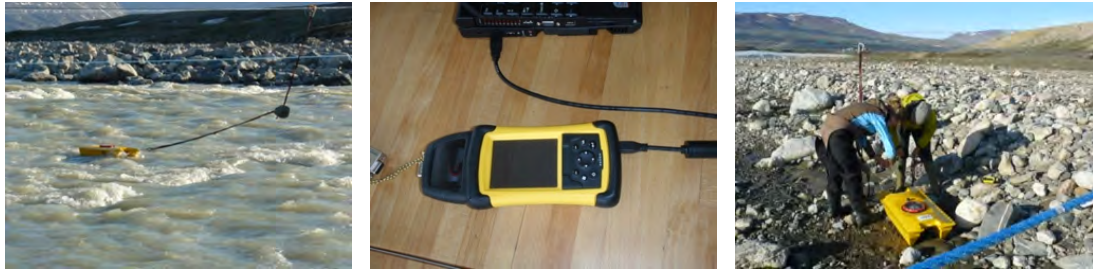
Figure 55: Q-liner boat in the river (left). PDA connected to computer (mid). Attaching the Qliner to the wire (right).
