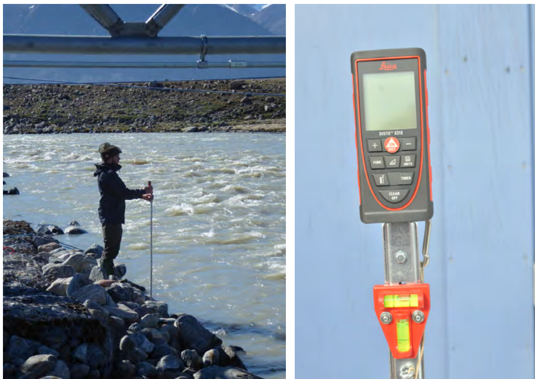
Figure 53: Measuring water table using the range finder and pointing it into the hoist trolley (left). Make sure the rangefinder is levelled using the small bobble level mounted on the pole (right)
