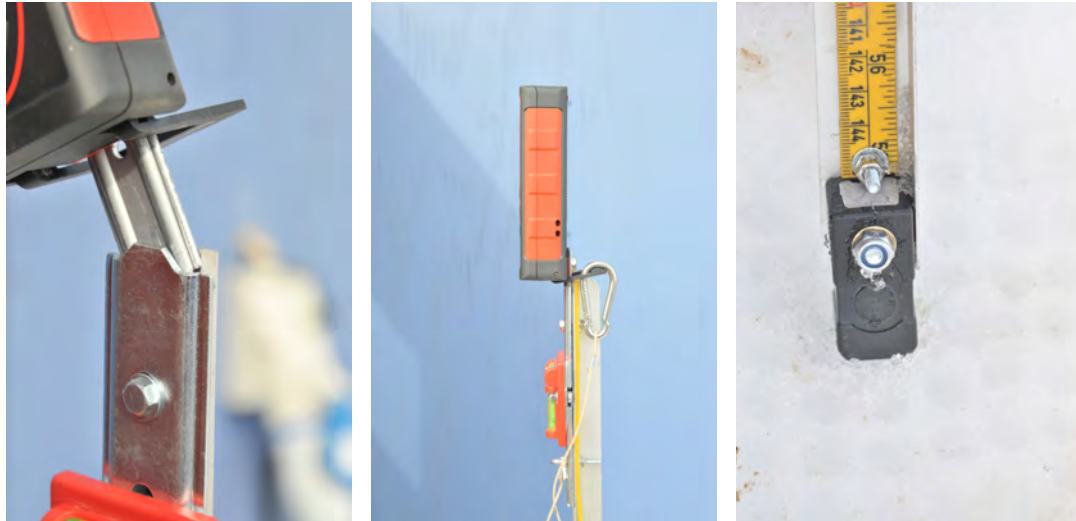
Figure 52: Correct mounting of range finder on pole with ruler (two leftmost photos) and placement of pole foot on a point directly under the hoist trolley (right photo).
