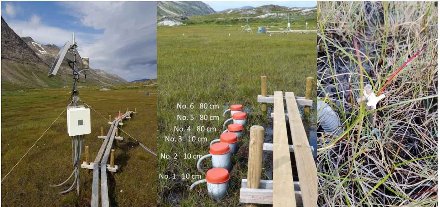
Figure 18 The automatic soil station SoilFen and the soil water sampling site close to the station.
