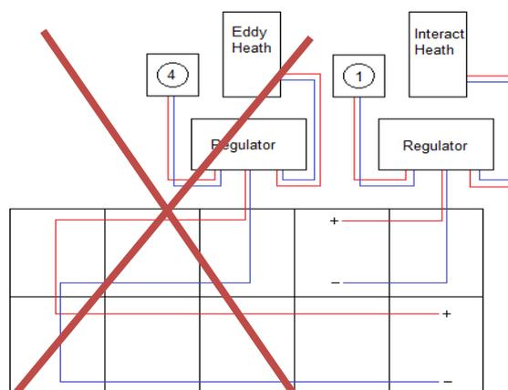
**Figure 28** Diagram of battery connection at the old setup.
