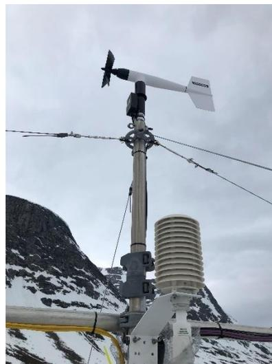
**Figure 16** Top: Young Wind sensor measuring wind speed and direction. Bottom: Air temperature and RH sensor (Vaisala, HMP155).
