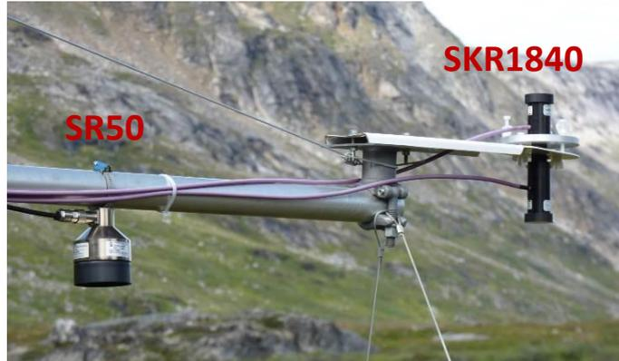
**Figure 15** Left: SR50 Snow Depth sensor, Right: NDVI sensor (Vegetation greenness).
