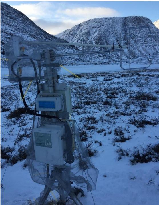
**Figure 21** Winter setup for the eddy station. Loggerboxes and cables are wrapped in fox net.
