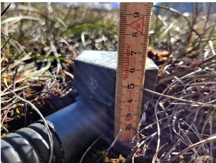
**Figure 17** SoilVUE10 sensor measuring soil temperature, moisture and conductivity.
