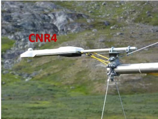
**Figure 14** Pyrano- and pygeometer (incoming and outgoing short- and long wave radiation).
