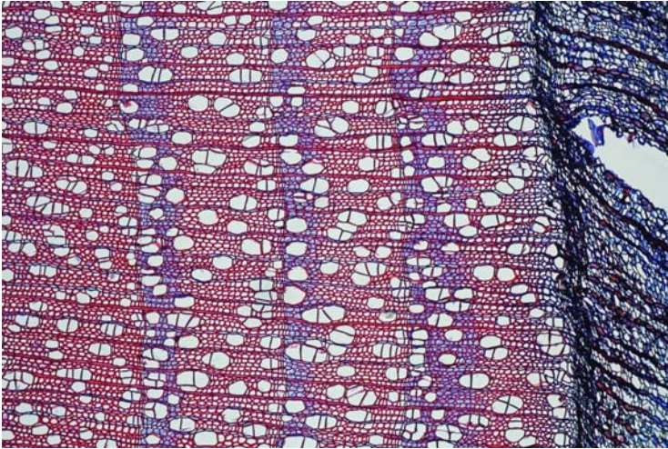
Figure 6.4 Three outer most rings and bark of Salix glauca and its cells and vessels. Blue parts are lignified (bark and tension wood) 6100x magnified. Photo: J. Lehejček.
