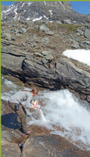
Discharge measurements using diluted salt in Kobbefjord. Photo: Asiaq.
