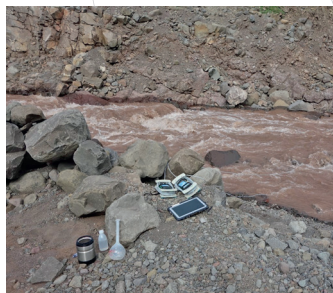
Discharge measurement using salt dilution in Chamberlin Stream, a tributary to Røde Elv in Disko, which carries meltwater and sediment from Chamberlin glacier. Photo: Asiaq.
