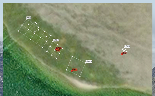
Figure 2. Updated georeferenced of the same plots. White dots are the points measured with RTK. Background image from Bing Aerial.
