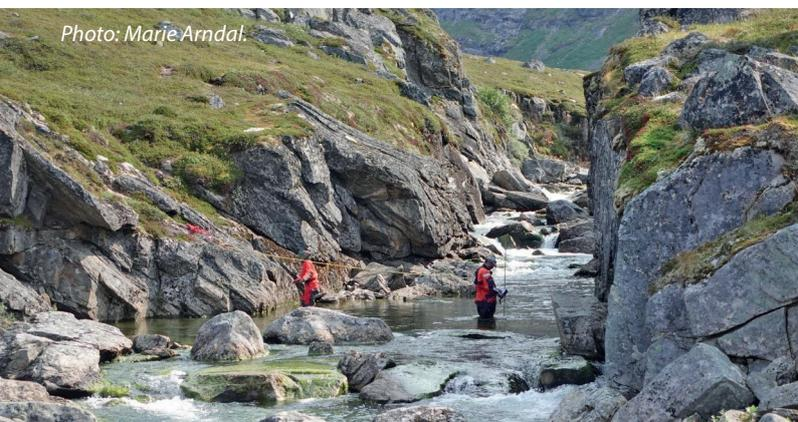
Discharge measurement using salt dilution, Kobbefjord. Photo: Asiaq.
