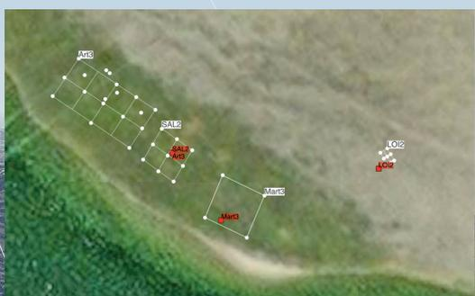
Figure 2. Updated georeferenced of the same plots. White dots are the points measured with RTK. Background image from Bing Aerial.
