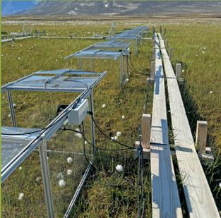
New chambers for methane and CO<sub>2</sub> flux monitoring installed at the fen in Zackenberg. Photo: Mikhail Mastepanov.
