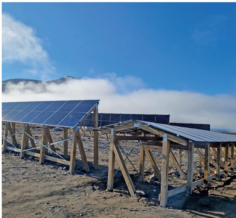
*Solar Panels in Zackenberg. Three configurations are being tested: 15° east/west, 45° south, and vertical 90° panels - both bifacial and monofacial - to assess performance under Arctic conditions and the midnight sun. The PV (photovoltaic) system was finalized in 2024. Photo: Marie Arndal.*
