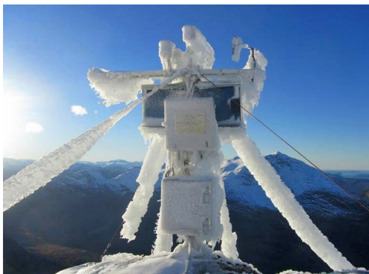
Figure 3.1 Micromet station, M1000, in March 2014 with heavy icing. The station was repaired in October 2013, but most sensors broke down less than two weeks later due to strong winds and heavy icing.
